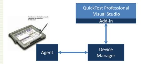
An agent is installed on the Windows CE device. The agent is responsible for the recording and the replay of the test commands The Device is connected to the PC using either WIFI, network or a USB connection. The Device Manager is the gateway between the connected devices and the extension inside QuickTest Profession or Visual Studio. The architecture allows the connection of multiple devices. One test script can execute against multiple devices.
